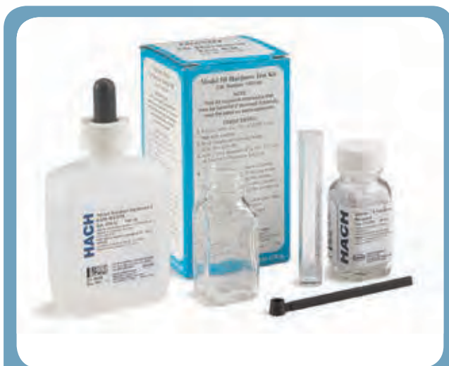
#49145300 hach 5b hardness test Kit 1 – 30 gpg Trust the original Hach test kit! Simple drop count Titration measures hardness as CaCo3 (1 gpg = 17.1 mg / l). 100 tests.
