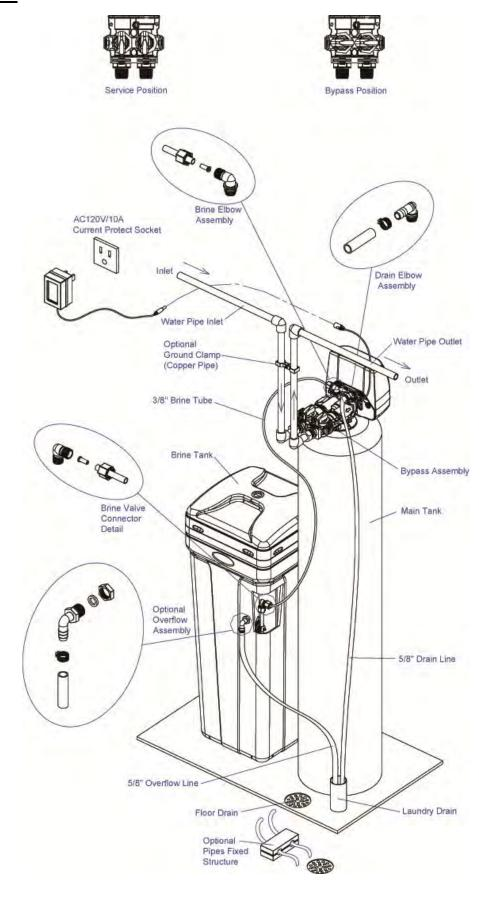
Note: As the picture shows, connect the inlet and outlet according to the arrow direction which seeing from the top view, where you can see the mark of "Up flow" or "Down flow" on the standard inlet and outlet connector assembly.
